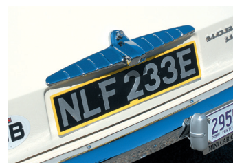
UK bootlid (left) had integrated number plate light and boot release.
