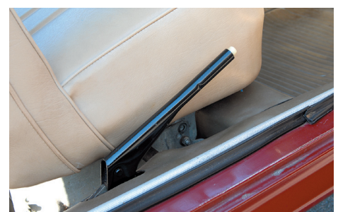
Handbrake moved to side of seat.
