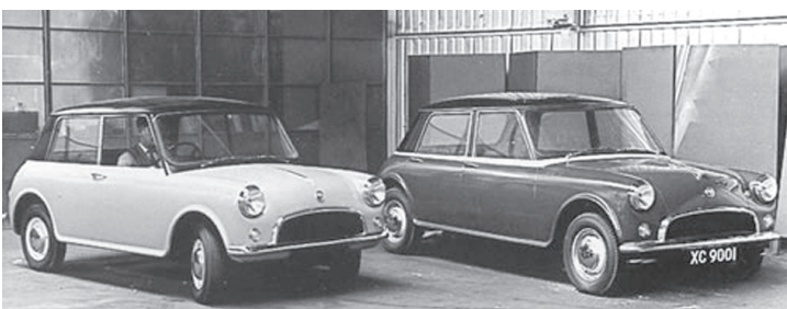
Front-wheel-drive XC9002 (left) and rear-wheel-drive XC9000.
